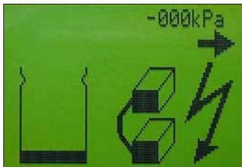
Fig. 32. Warning of short circuit between contact terminals, indicating position of short circuit (here: '→' means at contact terminals on right)
