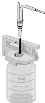
Fig. 7. Inserting the double connecting nipple
